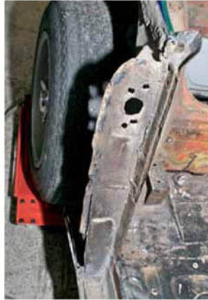
Clockwise from left Disassembly is started; typical rust on b-post; poorly repaired front yoke; repaired and patched frame, very common on Swedish cars.
