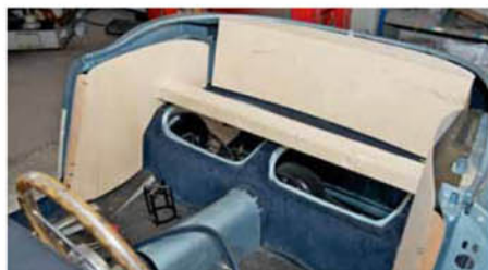
Above and below Custom made panels for doors, rear quarters and rear seat.
